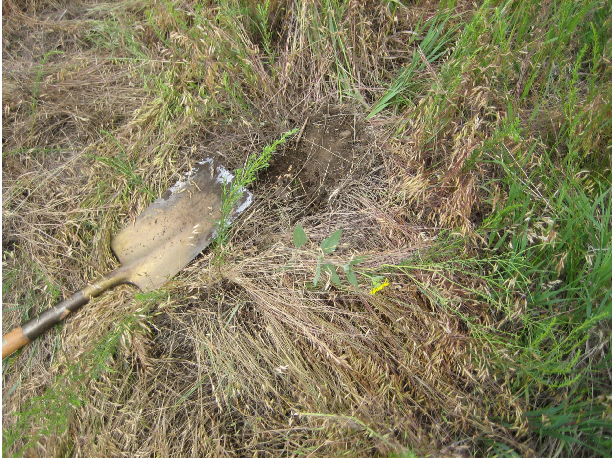
Figure 1. Process for collecting individual soil increments to 5 cm depths using a hand shovel.
