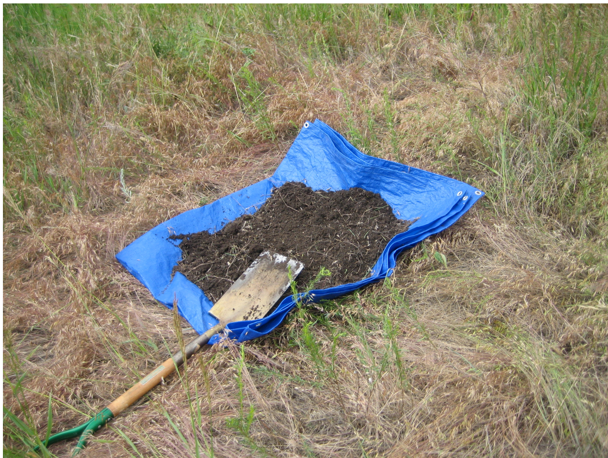
Figure 2. Example of a composite sample, obtained from one of the \sim 15\text{ m} \times 15\text{ m} plots, consisting of 25 – 30 shovels of soil. The material was blended and then a \sim 1\text{ kg} analytical aliquot was split in the field.
